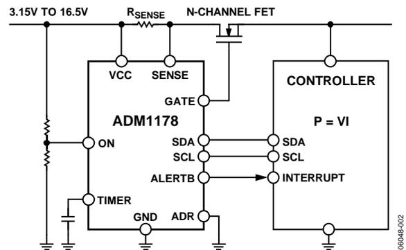
Figure 2. Applications Diagram
