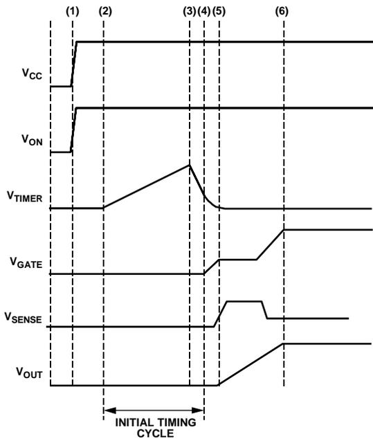
Figure 33. Startup (ON Asserts as Power Is Applied)
