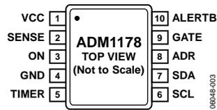
Figure 3. Pin Configuration
