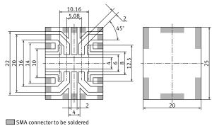
Connector (SMA type connector)
