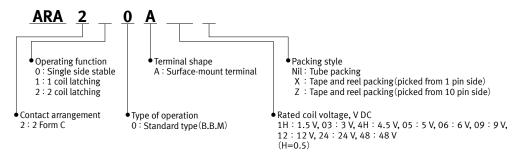
Notes: 1. 48 V coil type: Single side stable only 2. Packing style symbol "X", "Z" is not marked on the relay.
