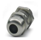
Cable gland, material for screw connection: Stainless steel 1.4305, application: Standard, external cable diameter 6 mm  $\dots$  12 mm, shielding: no, connecting thread: M20 x 1.5, color: silver, with O-ring
