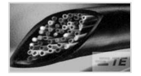
Primary Product Color: Black Wall Type: Single Wall Expanded Inside Diameter (Min): 19.1 mm [.75 in] Recovered Inside Diameter (Max): 10.9 mm [.429 in] Shrink Ratio: 1.75:1
