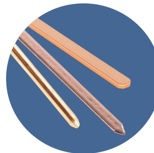
Our round heat pipes (not flattened) have a max temperature range of -40 C to 150 C. The heat pipe phase change benefits don't begin until you get to 10 C. Although 150 C is our max rated temperature we do recommend a max continuous use temperature of 130 C to help facilitate design integration.
