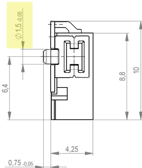
For the following article numbers we adapted the tolerance of the pig length: new 0,75mm - 0.1mm (old 0.75mm - 0.05mm)
