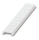
Zack Marker strip, flat, Strip, white, unlabeled, can be labeled with: PLOTMARK, CMS-P1-PLOTTER, mounting type: snapped, for terminal block width: 3.5 mm, lettering field size:  $3.5 \times 5.2 \text{ mm}$ , Number of individual labels: 10
