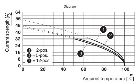
Derating curve for: PC 5/...-ST1-7,62 with PC 5/...-G-7,62 Conductor cross section: 6 mm<sup>2</sup>
