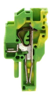
Feed-through terminal, Tension-spring connection, Mounting type: Plug in, Rated cross-section: 2.5 mm², Width: 5.1 mm, Colour: Green-yellow
