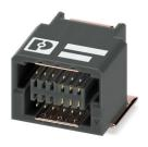
Shielded SMD female connector, nominal current: 1.7 A, Test voltage: 500 V AC, number of positions: 12, pitch: 0.8 mm, color: black, contact surface: Gold, contact connection type: Socket, mounting: SMD soldering
