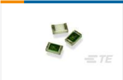
TE Part # 2-1614884-3 CPF 0805 18R 0.1% 25PPM 1K RL
