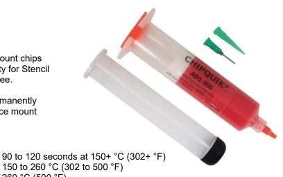
260 °C (500 °F) Designed to cure at leaded and lead free reflow temperatures. -40 to 125 °C (-40 to 257 °F) (After Curing, After Reflow) >15MPa (Steel-Steel, 25 °C (77 °F)) 1.25g/cc 450,000 mPa-s 80°C 60x10^-6/K (60 ppm/°C) 120x10^-6/K (120 ppm/°C) 0.14 W/(m·K) 25 KV/mm (at 25°C) 3.2 (at 25°C, 1MHz) <0.02 (at 25°C, 1MHz) <10% 30cc/30g Syringe Refrigerated >3 months, Unrefrigerated >3 months
