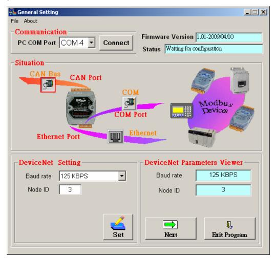
Step 8: Click the icon and in to configure the parameters of CAN bus (DeviceNet), COM port and Ethernet. For example, if you want to configure the CAN bus, click the icon of CAN bus. When you finish the configuration of DeviceNet on the frame of "DeviceNet Setting", click "Set" button. If configuration is successful, you can see the current configuration on the frame of "DeviceNet Parameters Viewer". After finishing all of the configuration, click "Next" button.
