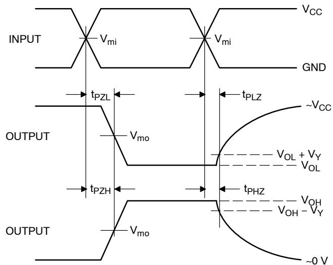
Figure 4. Switching Waveforms
