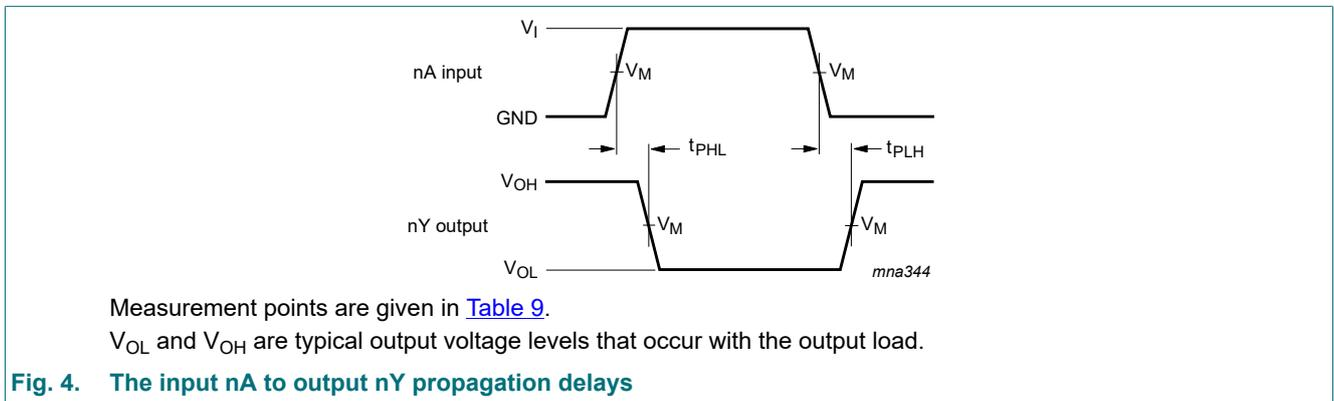
**Fig. 4. The input nA to output nY propagation delays**
