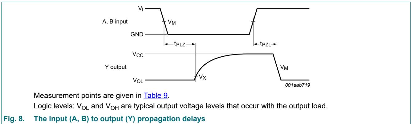
**Fig. 8. The input (A, B) to output (Y) propagation delays**
