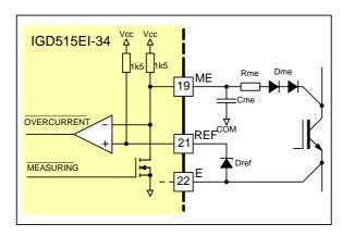
Fig. 4 Principle of V<sub>CE</sub> monitoring
