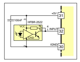
Fig. 7 Fiber-optic receiver wiring
