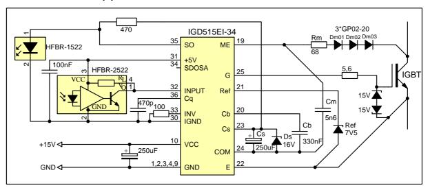
Fig. 9 Application example: Driving a 3300V/200A IGBT with IGD515EI-34
