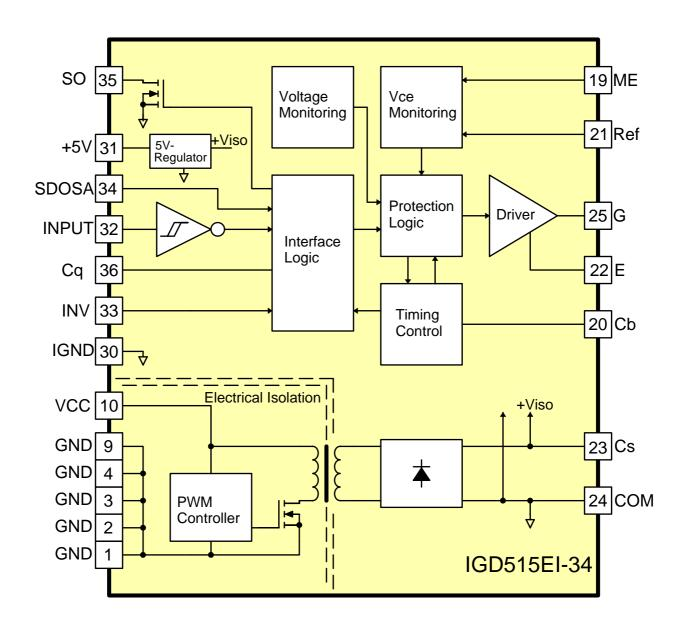
Fig. 1 Block and connection diagram of the IGD515EI-34
