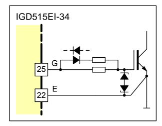
Fig. 3 Asymmetrical gate resistors
