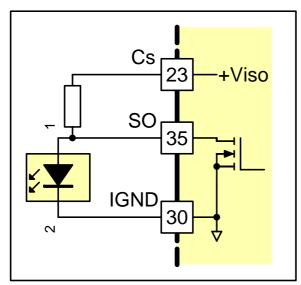
Fig. 8 Fiber-optic transmitter wiring voltage of about +15V is present here.
