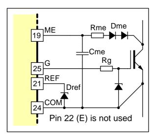
Fig. 6 Unipolar gate driving (0/+15V)
