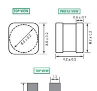
Recommended Soldering Pad Layout
