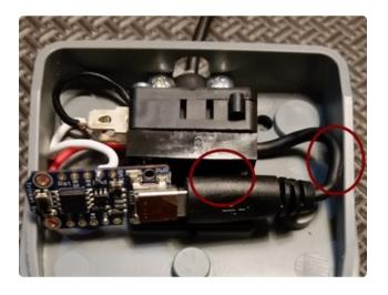
Tuck the Trinket and the cable up next to the switch. The top of the trinket board should not protrude above the switch so it will need to be placed at a slight angle. Put some pressure on the cable so the edge of the Trinket does not overlap the side of the pedal base.
