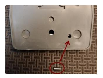
If you have the large hinge piece in and oriented correctly, then when you turn the foot switch over, the tiny pin will fit back in the hole shown. You might have to adjust the large pin back & forth a bit to get the tiny pin to fall flush with the back. If you inserted the large hinge pin backwards and the tiny pin does not fit, no worries, repeat the disassembly and reassembly steps.
