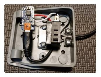
If you have not done so, strip 3/8" (3 millimeters) of insulation from the red and white wires. Solder the white wire to the GND pin on the Trinket. Solder the red wire to the #0 pin on Trinket.
