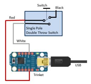
The wiring is shown above. The existing foot switch wires are cut short and two connected to Trinket pins #0 and GND (ground). When the foot switch is activated, the switch contact pair that creates a short connects Pin #0 with ground. When the Trinket detects the pin connected to ground, it outputs one or more characters as a PC keyboard.
