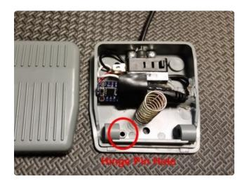
Here you can see the hot glue in place. When replacing the spring, it should not touch the Trinket. To be sure, I used a small piece of electrical tape.
