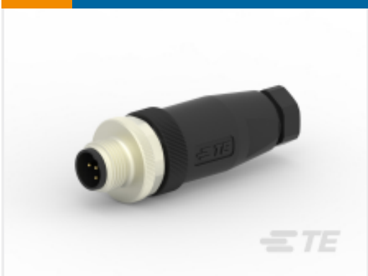
TE Part # T4111401051-000 M12,MALE,STRAIGHT,B CODE,5P, PG7,GOLD
