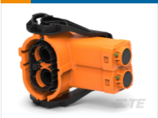
TE Part # 2-2286713-1 2POS,8MM HV,REC HSG,90DEG,ASSY, SEALED
