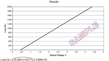
Sample Al-1000 calibration graph for a 2000 lb load cell
