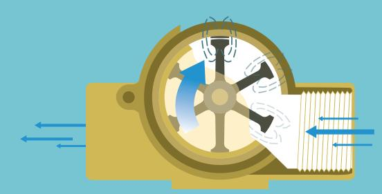
This flow meter is intended for high flow ranges from 19 L/min (5GPM) up to 114 L/min (30 GPM).
