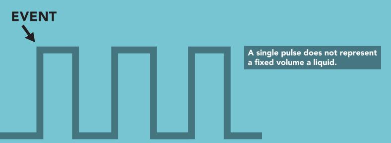
The amount of liquid moving through the flow meter is quantified by the frequency that the flow meter outputs. This is known as the flow meters K-factor.
