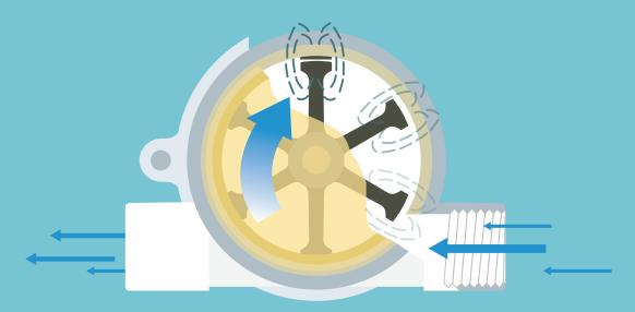
This flow meter is intended for low-to-medium flow ranges from 378 mL/min (0.09GPM) up to 19 L / min (5 GPM).
