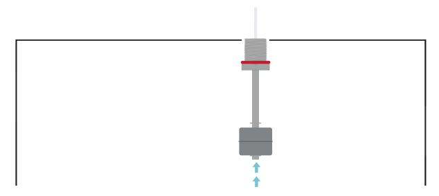
Now that the float switch is in place, re-attach and fully tighten the blukhead.
