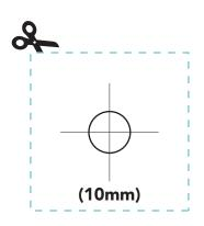
Once the (10mm) hole has been made, unscrew and remove the lock nut and o-ring. Install the float switch from the inside of your tank or contrainer.
