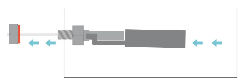
Now that the float switch is in place, re-attach and fully tighten the lock nut and o-ring.
