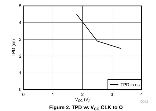
Figure 2. TPD vs  $V_{CC}$  CLK to Q
