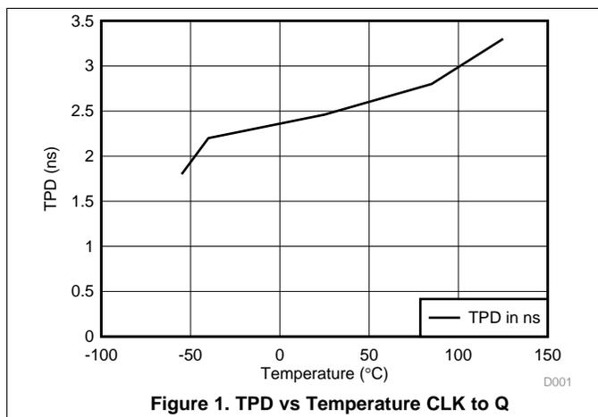
Figure 1. TPD vs Temperature CLK to Q
