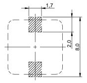
no sensitive traces underneath the component
