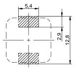
no sensitive traces underneath the component
