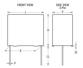
**General Information** Series PFR/F411 Dielectric Film/Foil Polypropylene Style Radial Features Pulse RoHS Yes Wire Leads Lead AEC-Q200 No Typical Component 0.386 g Weight An Operating Temperature Up To +105C Is Miscellaneous Allowed Under Certain Conditions. Please Consult KEMET For Details.
