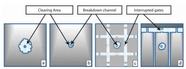
a and b: not segmented metallization;
