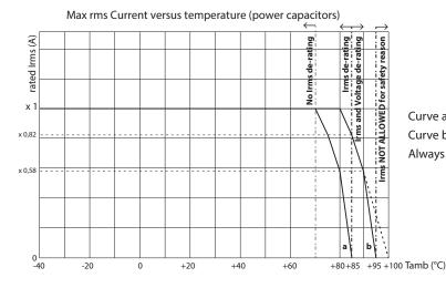
Curve a: DCB, DCS, PHC, RHB, RMC, PPS, PPA, RSB, RMB, MAR. Curve b: other series for power applications.
