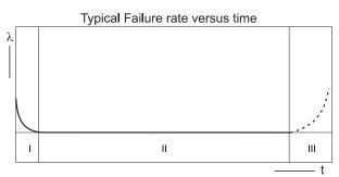
Failure rates data at specifications are typically referred to the second period (II) only.
