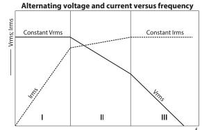
I: area where voltage is limited by ionization
