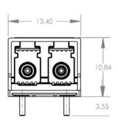
Measurements are in mm
