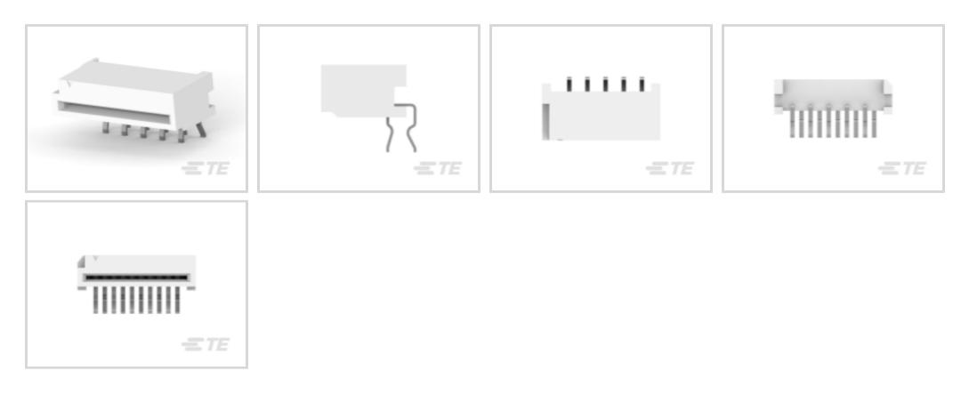
Connector System: Flex-to-Board Number of Positions: 10 Centerline (Pitch): 1.25 mm [.049 in ] Insertion Force Type: Non-ZIF PCB Mount Orientation: Right Angle
