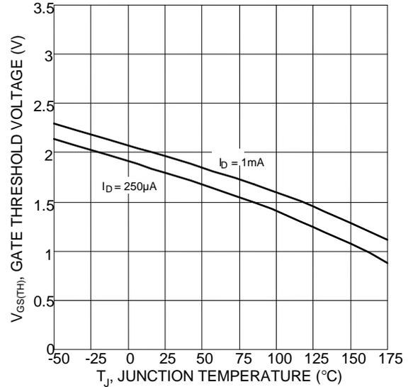
Figure 8 Gate Threshold Variation vs. Junction Temperature
