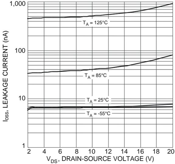
Fig. 11 Typical Leakage Current vs. Drain-Source Voltage
