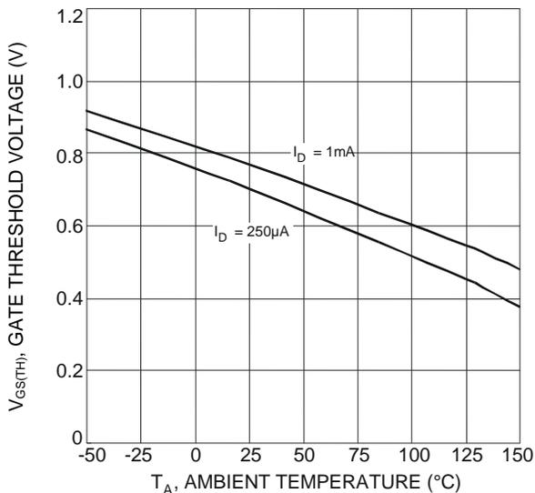
Fig. 9 Gate Threshold Variation vs. Ambient Temperature
