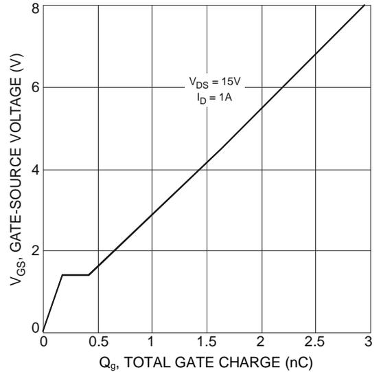
Fig. 14 Gate-Charge Characteristics
