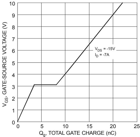
Figure 23 Gate-Charge Characteristics
