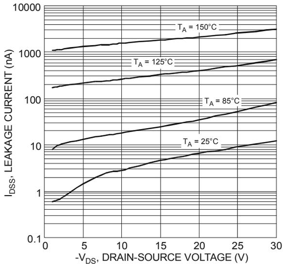
Figure 21 Typical Drain-Source Leakage Current vs. Voltage
