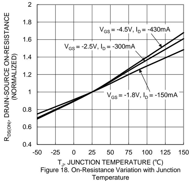
Figure 18. On-Resistance Variation with Junction Temperature
