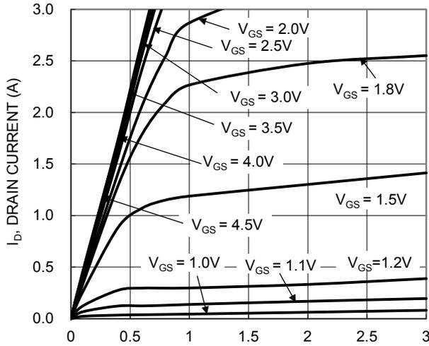
$V_{DS}$ , DRAIN-SOURCE VOLTAGE (V)
