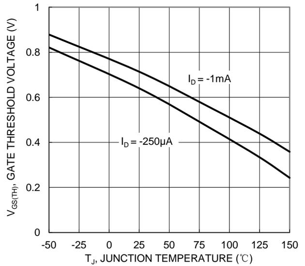
Figure 20. Gate Threshold Variation vs. Junction Temperature
