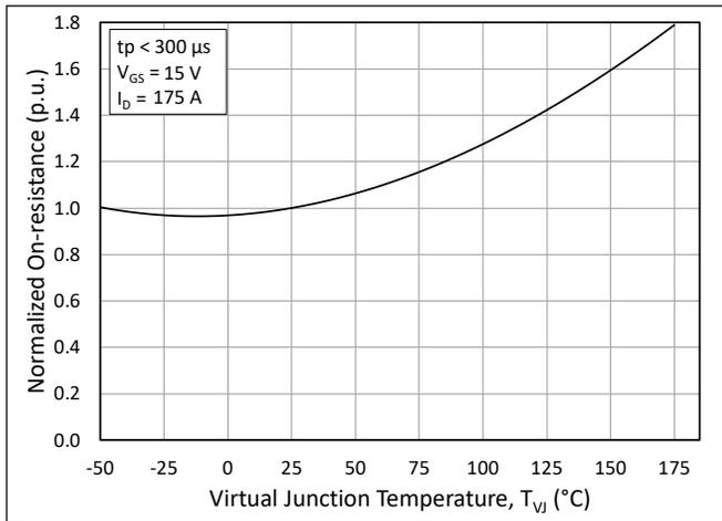
Figure 3. Normalized On-State Resistance vs. Junction Temperature
