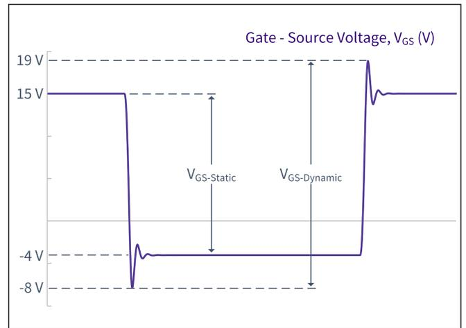
**Figure 33. V<sub>GS</sub> Transient Definitions**
