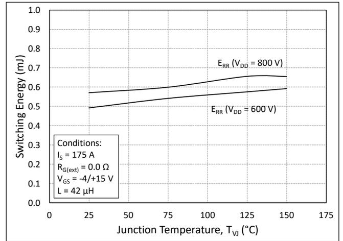
Figure 14. Reverse Recovery Energy vs. Junction Temperature
