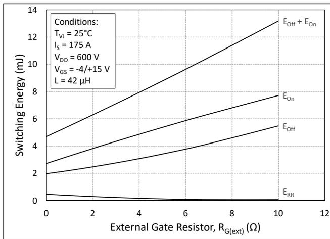
Figure 15. MOSFET Switching Energy vs. External Gate Resistance
