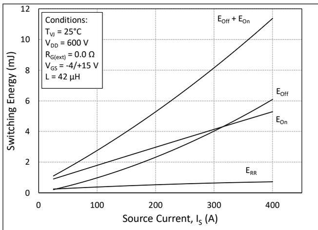
Figure 11. Switching Energy vs. Drain Current ( $V_{DS} = 600$  V)
