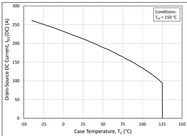
Figure 21. Continuous Drain Current Derating vs. Case Temperature
