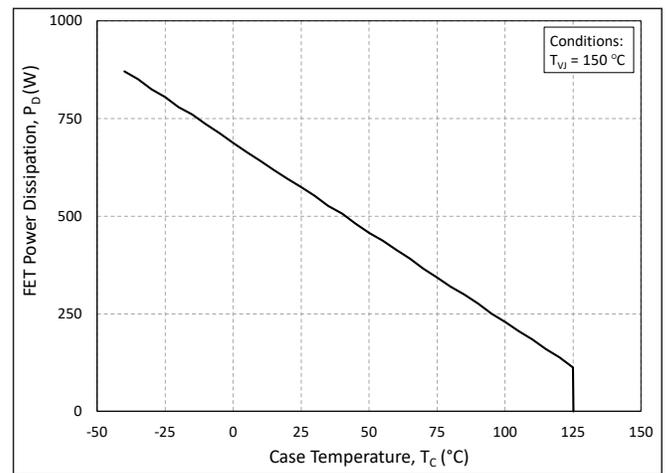
Figure 22. Maximum Power Dissipation Derating vs. Case Temperature
