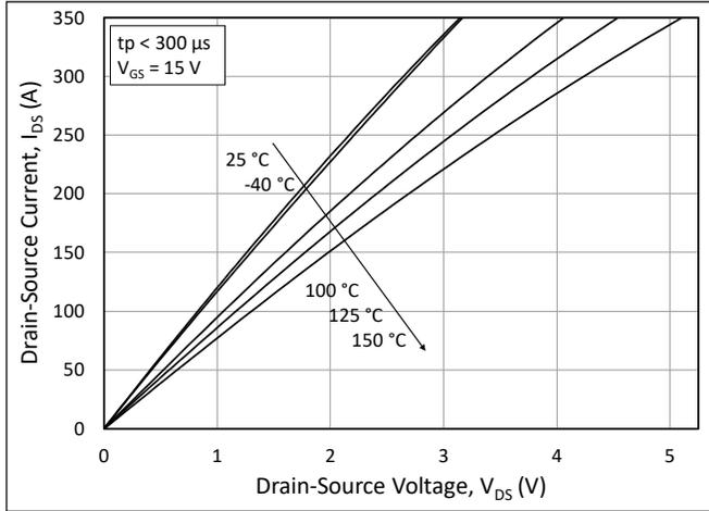
Figure 1. Output Characteristics for Various Junction Temperatures
