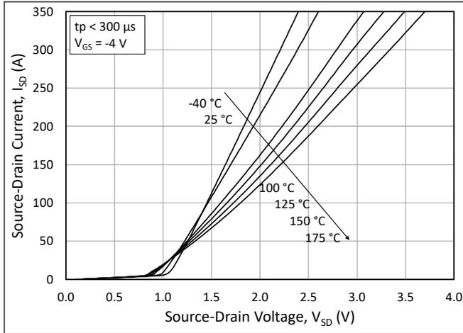
Figure 7. 3<sup>rd</sup> Quadrant Characteristic vs. Junction Temperatures at  $V_{GS} = -4$  V (Diode)
