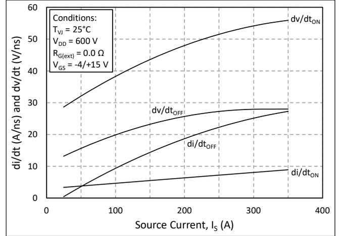
Figure 25. dv/dt and di/dt vs. Source Current
