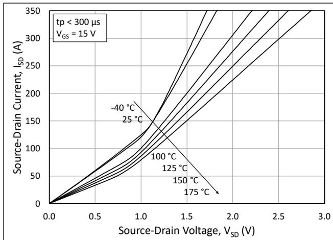
Figure 5. 3<sup>rd</sup> Quadrant Characteristic vs. Junction Temperatures at  $V_{GS} = 15\text{ V}$
