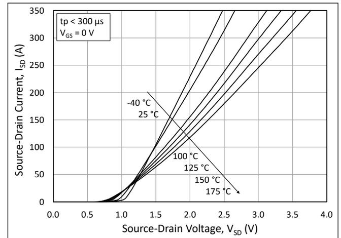
Figure 6. 3<sup>rd</sup> Quadrant Characteristic vs. Junction Temperatures at  $V_{GS} = 0\text{ V}$  (Diode)
