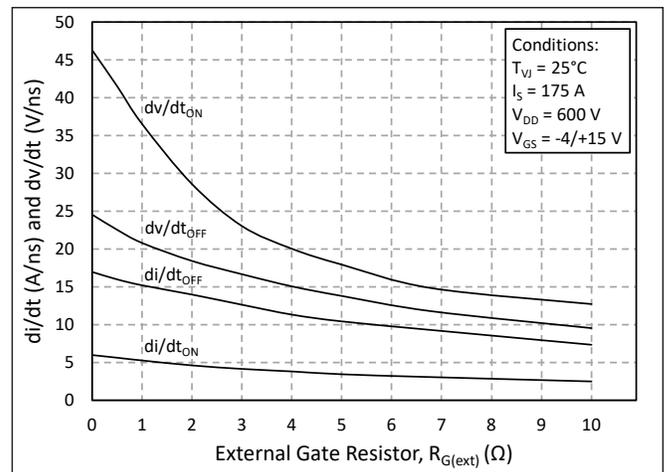
Figure 29. dv/dt and di/dt vs. External Gate Resistance
