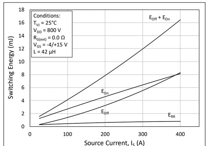
Figure 12. Switching Energy vs. Drain Current ( $V_{DS} = 800$  V)
