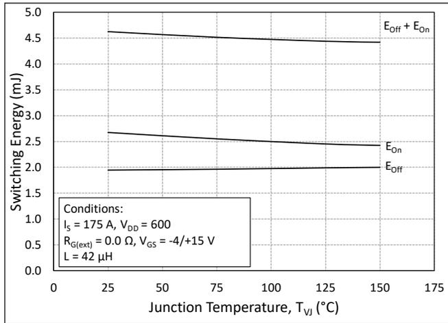
Figure 13. MOSFET Switching Energy vs. Junction Temperature
