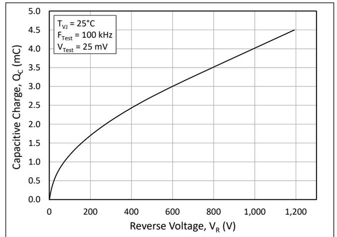
Figure 4. Typical Capacitive Charge vs. Reverse Voltage
