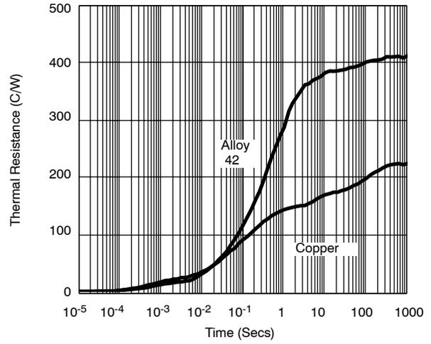
**FIGURE 5.** Dual SC70-6 Comparison on 1-inch<sup>2</sup> PCB
