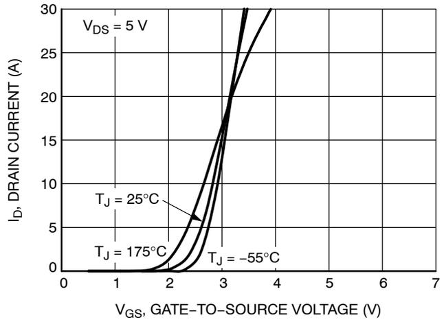
Figure 2. Transfer Characteristics
