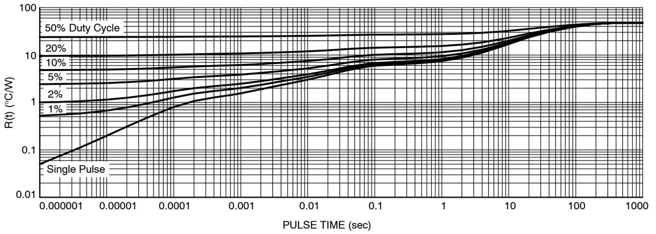
Figure 13. Thermal Characteristics
