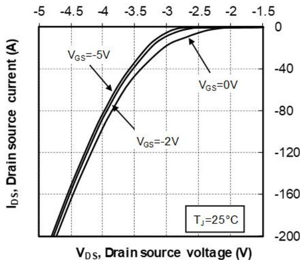
Figure 1-11. 3<sup>rd</sup> Quadrant Characteristics,  $T_J = 25^\circ\text{C}$
