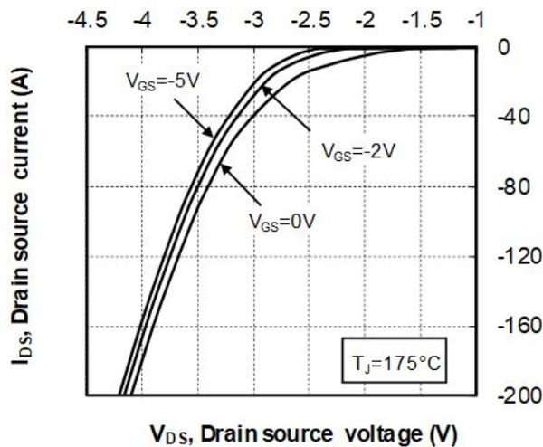
Figure 1-13. 3<sup>rd</sup> Quadrant Characteristics,  $T_J = 175^\circ\text{C}$
