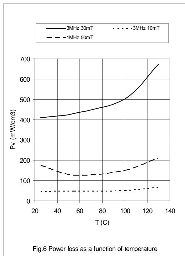
Fig.6 Power loss as a function of temperature
