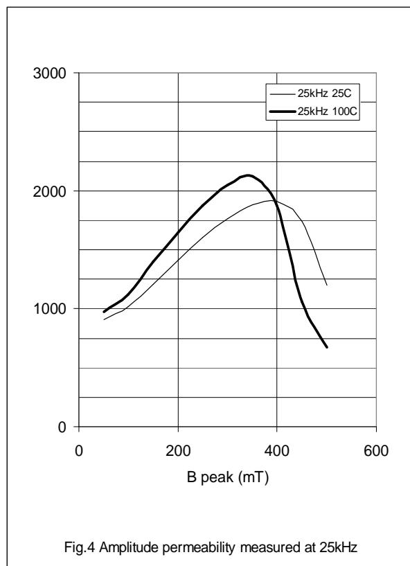
Fig.4 Amplitude permeability measured at 25kHz
