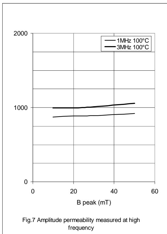
Fig.7 Amplitude permeability measured at high frequency
