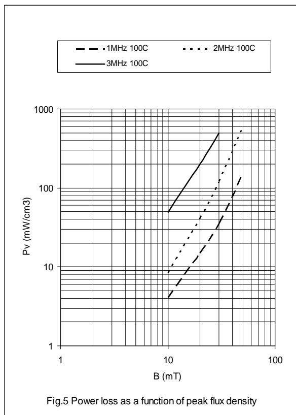
Fig.5 Power loss as a function of peak flux density
