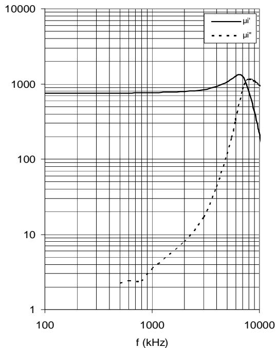
Fig.1 Complex permeability as a function of frequency
