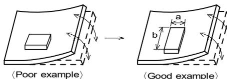
(2) Components location on PCB separation
