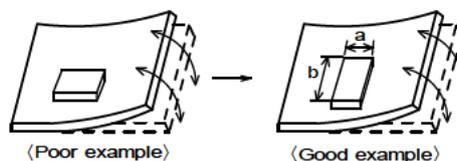
(2) Components location on PCB separation
