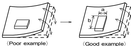
(2) Components location on PCB separation
