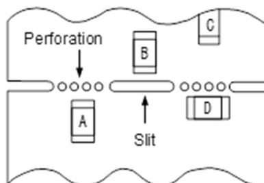
**(3) Mounting components near screw holes**
