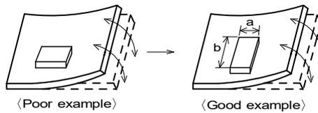
(2) Components location on PCB separation
