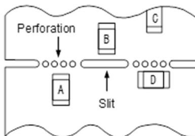
(3) Mounting components near screw holes
