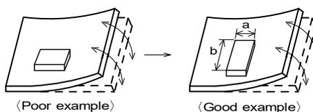
(2) Components location on PCB separation
